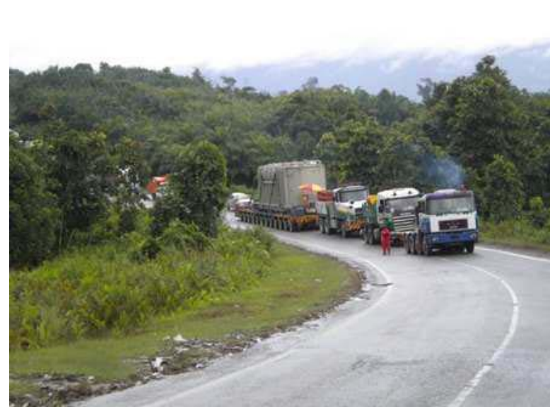
Transporting a Power Transformer up hilly terrain to the Bakun Hydroelectric Power Station site at Sarawak, Malaysia.
